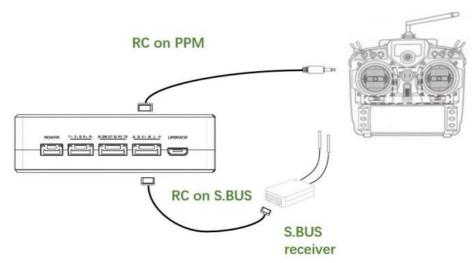
Using PPM mode: Insert the training connector of the supplied RC cable to the training port of a remote controller and connect the six-pin connector of the RC cable to the RC port of the ground unit.
