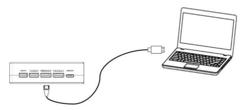
Insert the six-pin connector of supplied serial cable to the serial port of the ground unit and connect the other end of supplied serial cable to the telemetry port of the ground control station.
