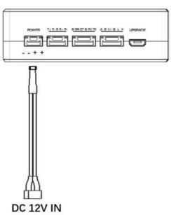
Pin-out: - - + +. Insert the four-pin connector of supplied power cable to the power port of the air unit and connect the orange power connect of supplied power cable to a battery output, or the power supply port of a drone. Recommended voltage is 12V.
