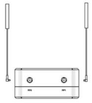
Insert the air unit antennas into the RF ports. Antenna clicks in when properly installed.
