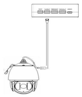
Connect the ethernet video output port to the ethernet video input port of the air unit.
