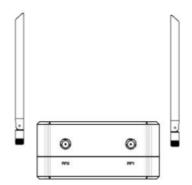
Insert the air unit antennas into the RF ports with RF cables. RF cables clicks in when properly installed.
