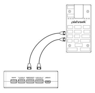
Insert the six-pin connector of supplied serial cable to the serial port of the air unit and connect the other end of the serial cable to the telemetry port of a flight controller.
