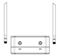
Insert the air unit antennas into the RF ports with RF cables. RF cables clicks in when properly installed.
