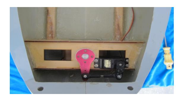
Install servo for nose gear
