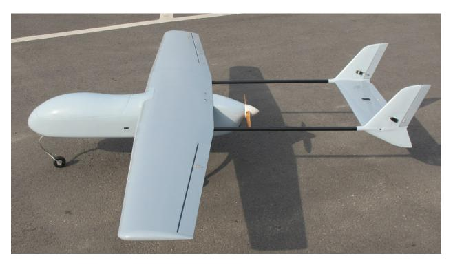
Wingspan: 2600mm Length: 2020mm
